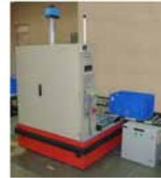
(left) Four Piece Servo Manipulator for existing hotcells
